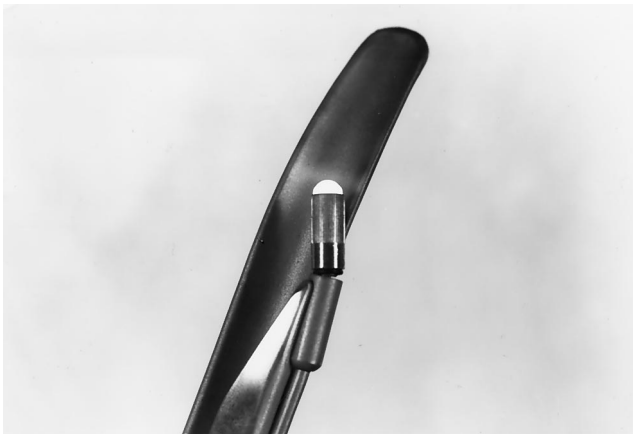
Figure 1. Miller 3 laryngoscope blade with functional bulb fractured at the base.
